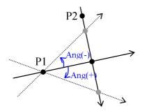
In the O/S field, enter a positive value to specify an offset to the right. Enter a negative value to specify an offset to the left.
