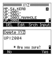
You can also delete coordinate data by pressing the DEL softkey in the detailed display screen for the record.
