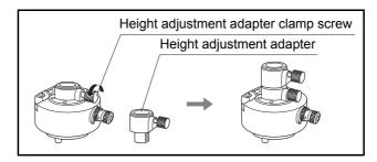
The height adjustment adapter will be removed when used with the Nivo series instrument.
