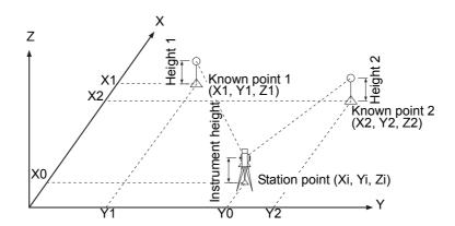
You can use a maximum of 10 points in a resection. Measurements can be distance and angle, or angle only. Calculation starts automatically when enough measurements are taken.
