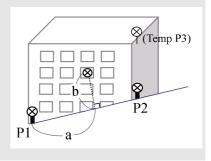
Once the plane is defined, the calculated a and b values are updated as you move the telescope. No distance measurement is required.
