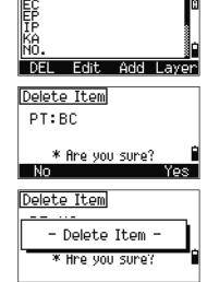
To delete a whole layer, highlight the layer name in the list and press the DEL softkey. All codes and layers in the selected layer are deleted.
