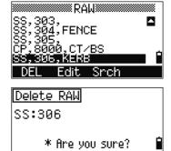
If the Store DB setting is set to Both, the system also deletes the corresponding coordinate data when you delete an SS, SO, or CP record.
