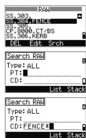
To search by point type, move to the Type field and use < or > to change the selected point type. The options are ALL, ST, SS, SO, CP, CO, CO(SY), and CO(RDM).
