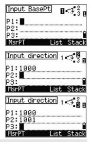
When you press the MSR softkey, a temporary measuring screen appears. Sight the target and press [MSR1] or [MSR2] to take a measurement.
