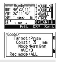
In Quick code measurement, the Rec mode can only be set to Confirm or ALL.
