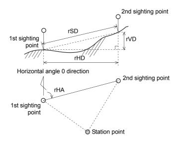
rSD Slope distance between two points rHD Horizontal distance between two points rVD Vertical distance between two points rV% Percentage of grade (rVD/rHD) × 100% Vertical grade (rHD/rVD):1 rGD rAZ Azimuth from first point to second point
